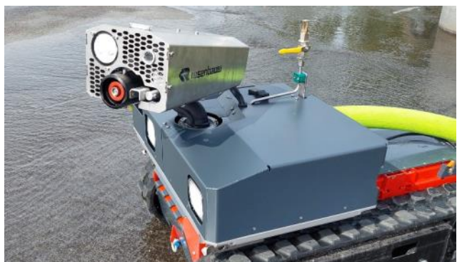
CC81G-A101 - module RM15C (up to 2.000 l/min at 10 bar)
