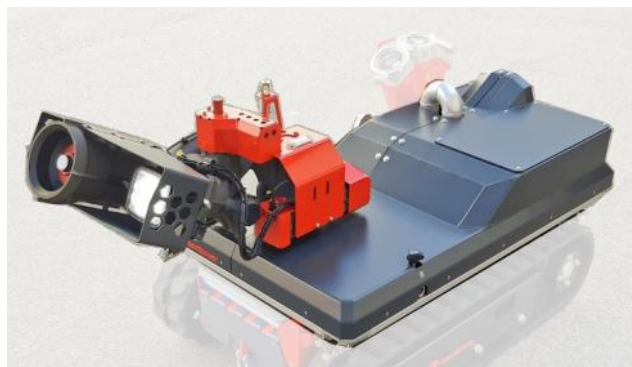
CC81J-A101 - module RM35C (up to 3.800 l/min at 10 bar)
