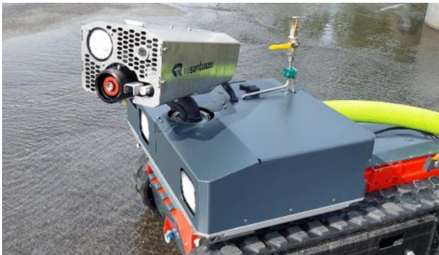
CC81G - module RM15C (up to 2.000 l/min at 10 bar)
