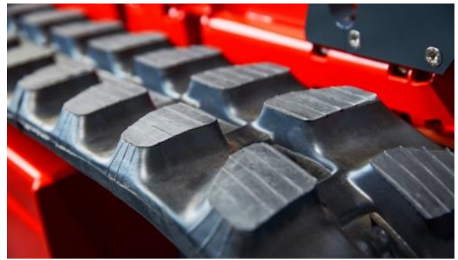
Rubber chains with 150 mm width for good traction
