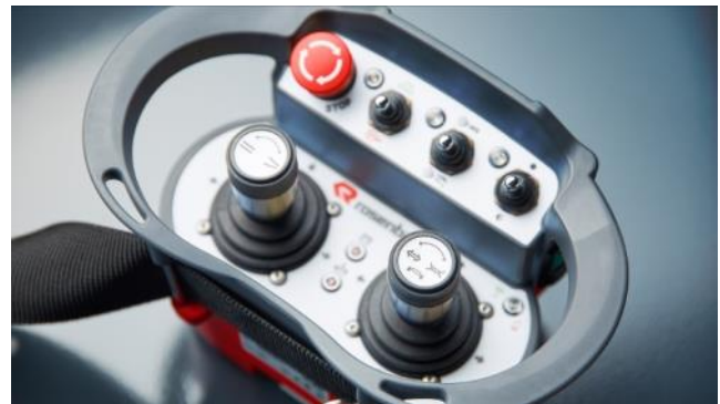
T3 with 2 joysticks - for Robot chassis and f.e. turret
