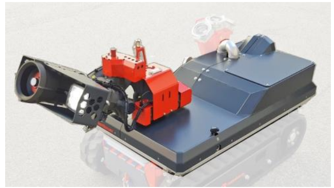
CC81J - module RM35C (up to 3.800 l/min at 10 bar)
